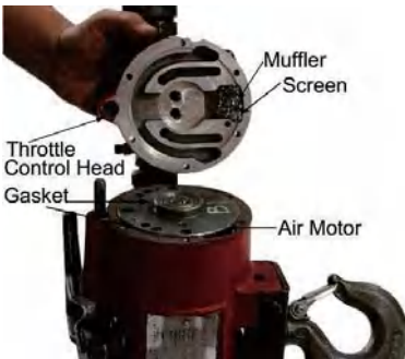
Figure 13 -Removing Control Head Assembly
