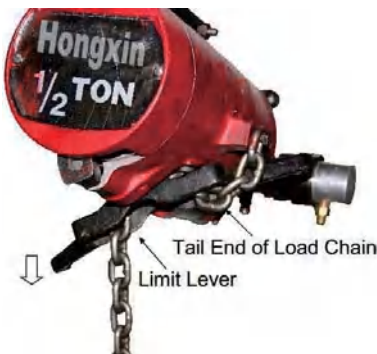
Figure 6 -Control Lever Being Tripped by Tail End of Load Chain
