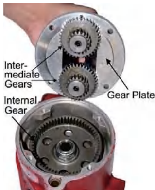
Figure 17 -Removing Gear Plate and Intermediate Gears
