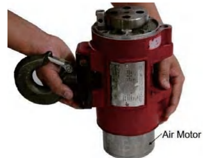
Figure 14 -Removing Motor from Frame
