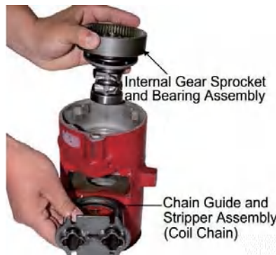
Figure 18 -Removing Internal Gear, Chain Sprocket and Ball Bearing Assembly
