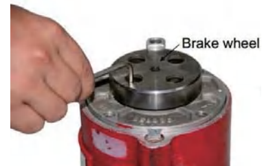
Figure 15 -Removing Cap Screws Securing Bearing Clamp Plate
