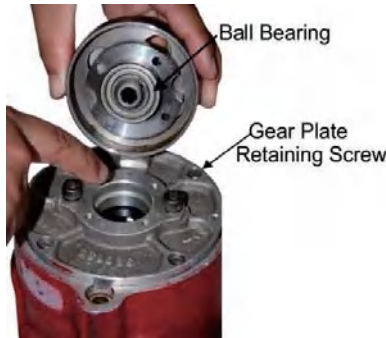
Figure 16 -Removing Brake Wheel and Ball Bearing Assembly
