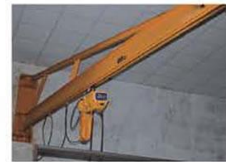
悬臂吊 Jib Crane
